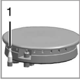
1. Gas shut off safety
